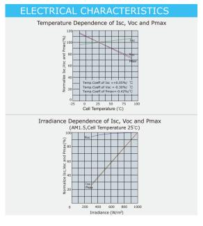
**Note:** the specifications are obtained under the Standard Test Conditions (STCs): 1000 W/m² solar irradiance, 1.5 Air Mass, and cell temperature of 25°C. The NOCT is obtained under the Test Conditions: 800 W/m², 20°C ambient temperature, 1m/s wind speed, AM 1.5 spectrum.
